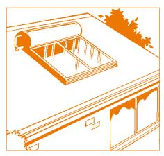
This circular heating motion is called the 'thermosyphon effect'. The greater the difference in temperature between the water in the collectors and the water in the storage tank, the faster the flow between them. A closed circuit system separating the collector circuit from the tank is available for areas prone to frost or hard water (e.g. water from groundwater bores).
