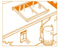
The pump is regulated by a controller, which reacts according to the difference in water temperature between the collectors and the tank.
